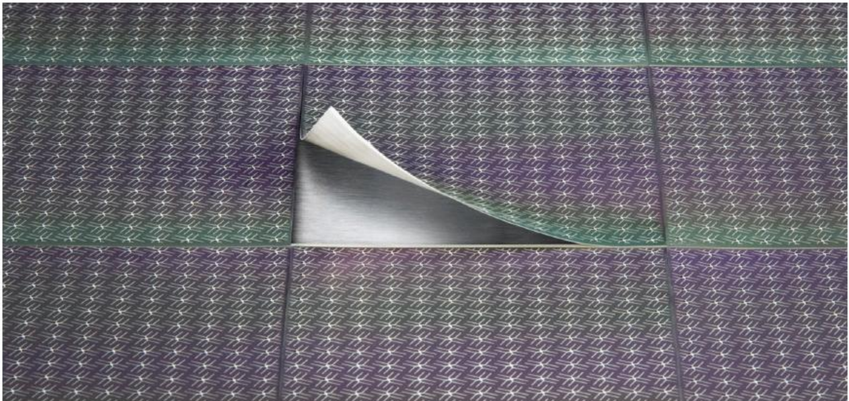
Figure 15: Nanosolar MWT back-contact cells are interconnected into electrical circuits via tabs on each cell that are simply the overhang of one of the two laminated aluminum foils.
