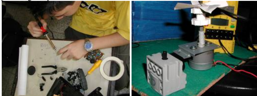
Figure 4 - A student disassembles the tape recorder (left), the expensive Lego motor, and the motor salvaged from the tape recorder (right)
