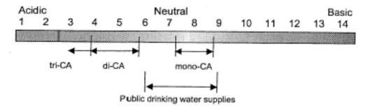
Chloramines are formed as a result of the reaction between added chlorine and ammonia naturally present in the water or ammonia that has been deliberately added so that a combined chlorine residual will be formed.
