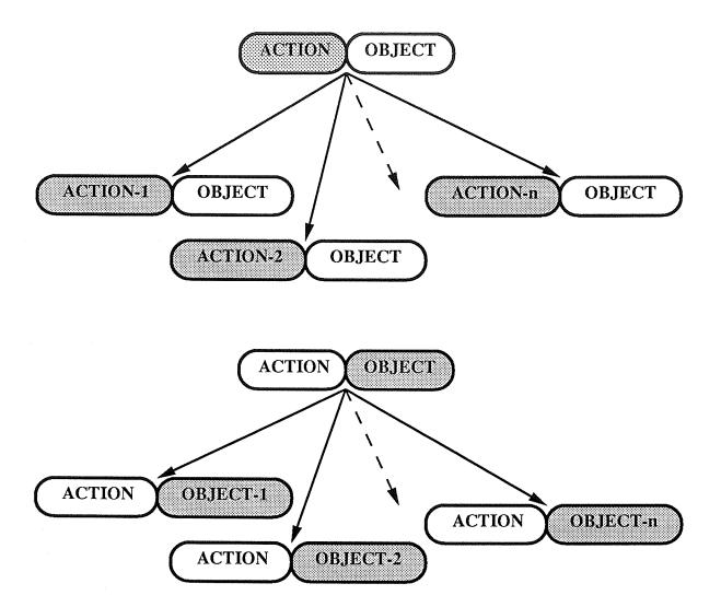
Figure 3. Activity Elaboration by Scale Reduction: The scale of an activity is a function of the scale of its constituents. Thus, to reduce the scale of an activity, the scale of an action or that of an object is reduced. The scale of an action is reduced along the 'elaborates-to' relation. The scale of an object is reduced along several relation such as 'sub-part' and 'containts'.
