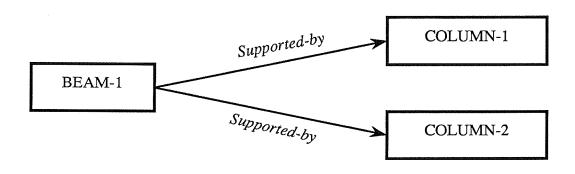
Figure 4. Supported-By Relation: The 'supported-by' relation is one of the main relations that forces precedence constraints between activities that have facility components as objects. This relation exemplifies the type of information that OARPLAN would get by posing a high level query to a database interfaced with a CAD system.
