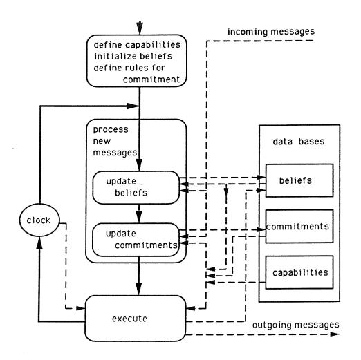
Figure 2: A flow diagram of AGENT0's interpreter
