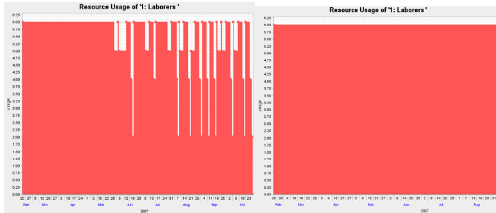
Figure 5: GAPO improves the resource leveling of the resource Laborers within 10 seconds from the initial schedule (as shown on the left graph) to its final Pareto optimal schedule (as shown on the right graph). This suggests that the algorithm has a short latency to find the Pareto optimal decision alternative combinations.
