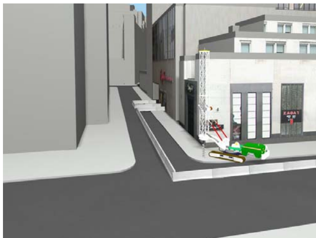
Figure 26: Dey Street Piling Sequence Stage 4, in front of Century 21
