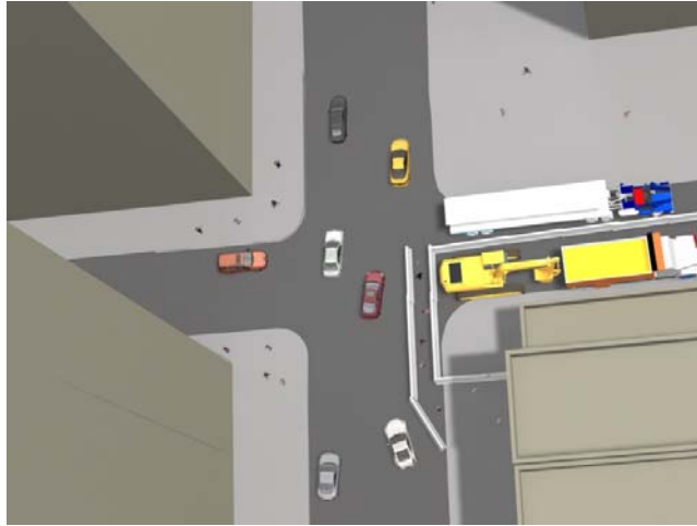
Figure 9c: Rendering of construction stage 3 of the 4/5 Southern Entrance. Work-zone in S-E corner of street.
