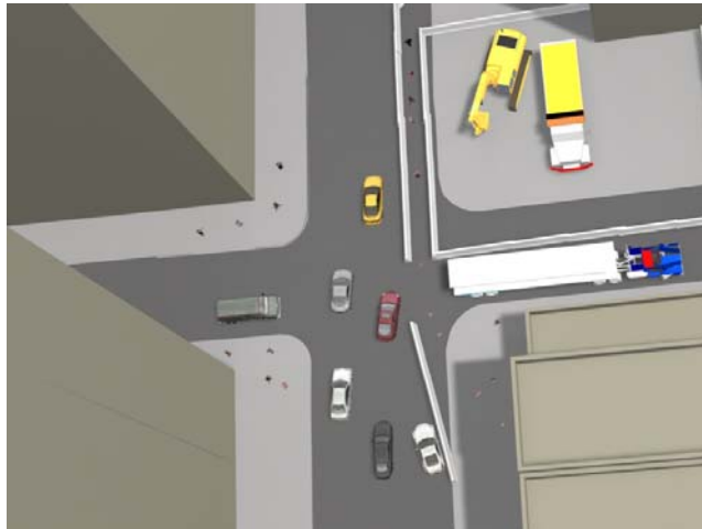
Figure 9b: Rendering of construction stage 2 of the 4/5 Southern Entrance. Work-zone in N-E corner of street.
