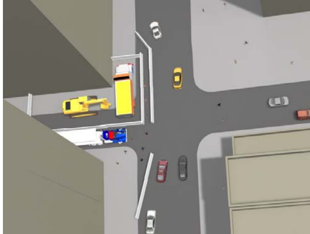
Figure 10a: Rendering of construction stage 1 of the 4/5 Southern Entrance. Work-zone in N-W corner of street.
