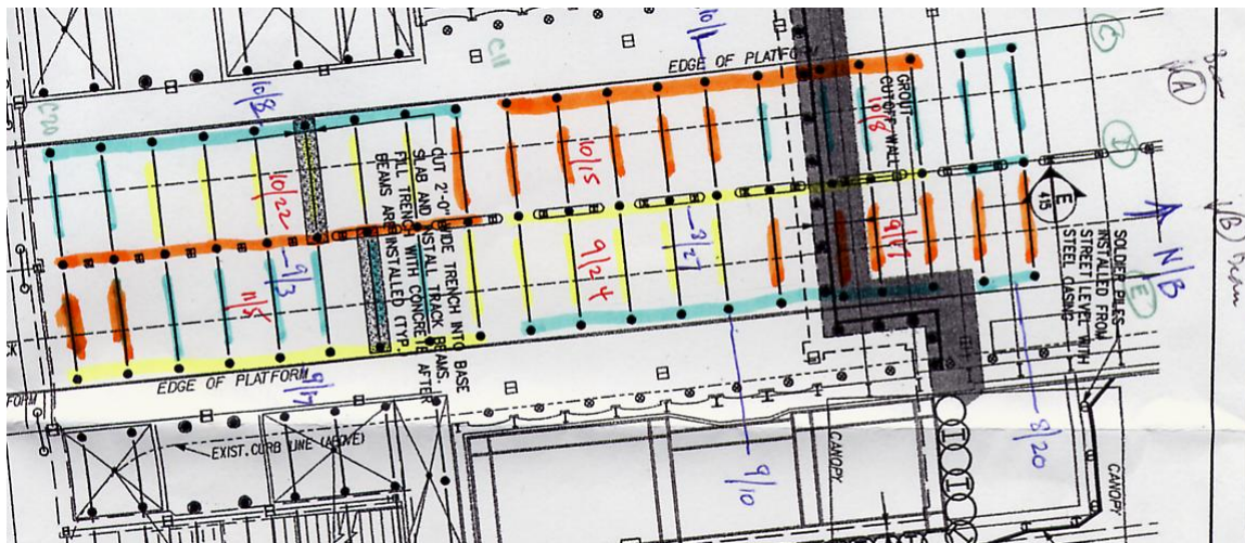
Figure 20 - Marked up 2D drawing of the scheduled piling sequence
