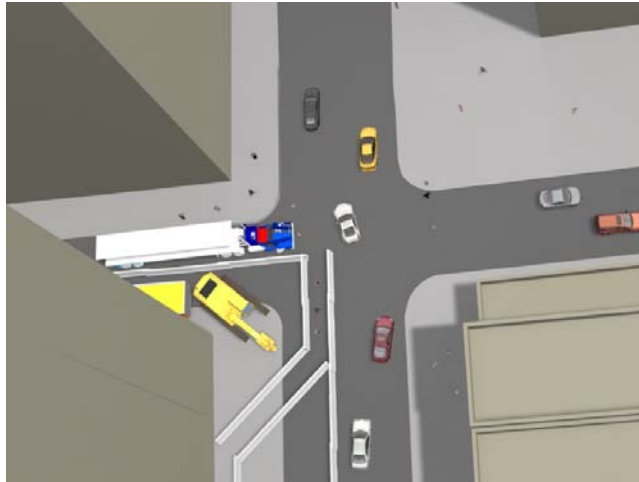
Figure 9d: Rendering of construction stage 4 of the 4/5 Southern Entrance. Work-zone in S-W corner of street.
