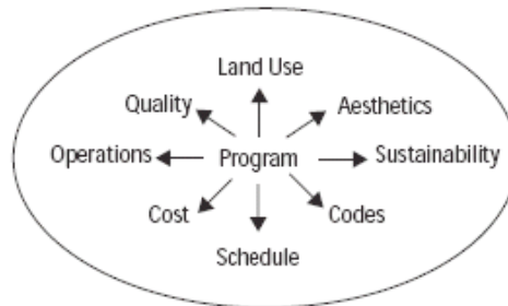
Fig. 2. Diagram by a university owner identifying the tradeoffs required for the design of its buildings. The relative importance of Goals is rarely quantified in AEC projects today.
