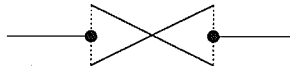
Figure 14: Port attachment points ideally should be constrained to specific primitives used to define a drawing symbol. The present interpretation algorithm does not constrain any entity ports to specific symbol primitives.
