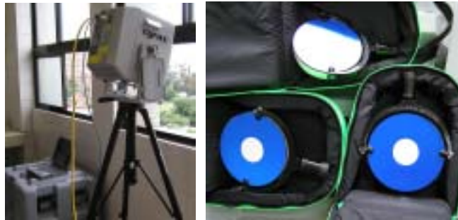
Figure 1. Cyrax 2500 3D laser scan system and registration points
