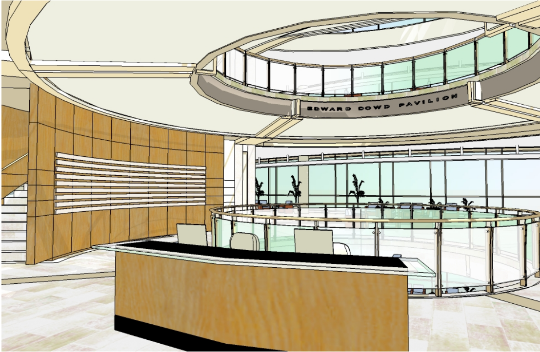
Figure 4: A 3D rendering of the interior of the lobby of the Camino Medical Group Project. The rendering was developed in the early Schematic Design phase to communicate the finishes in the lobby to the owner. Image courtesy HPS Architects, Mountain View, CA, USA.
