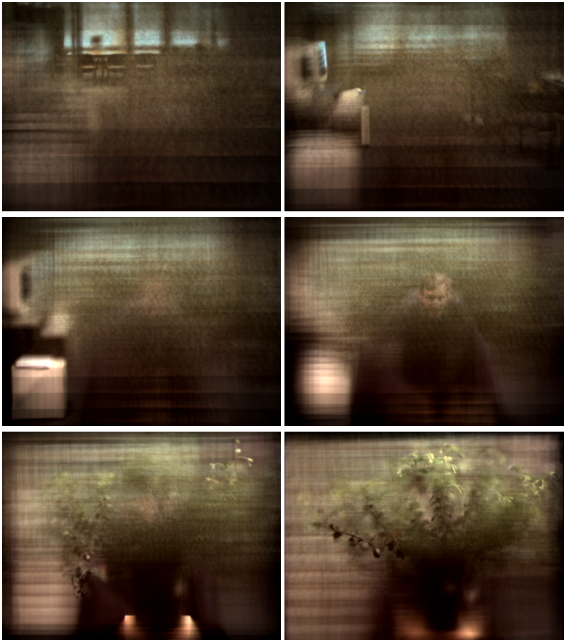
Figure 4.10: Sweeping the synthetic aperture focal plane. In this sequence of synthetic aperture images, the focal plane is swept toward the camera array. Objects visible at one focal depth disappear at others, allowing us to clearly see the person hiding behind the plant, even though he was mostly occluded in the input images.
