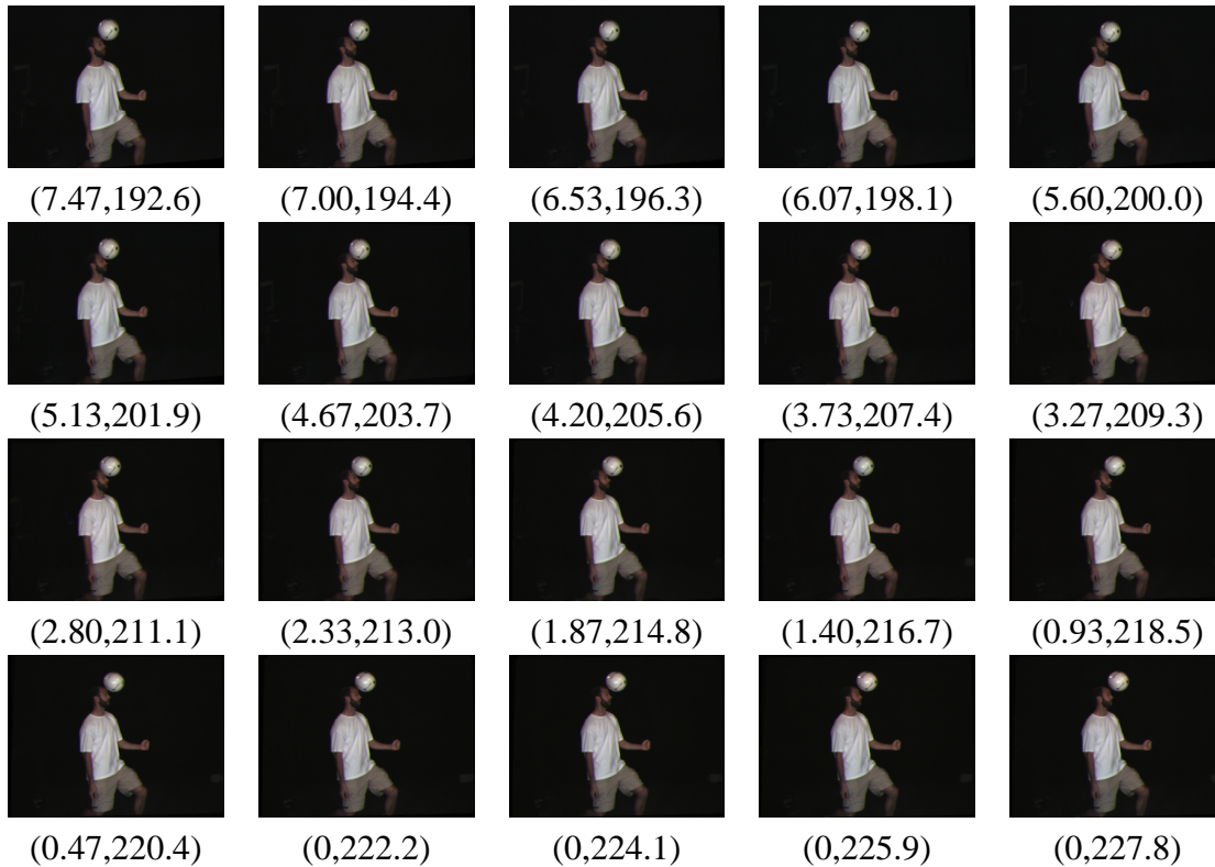
Figure 6.6: Twenty sequential frames from an interpolated video sequence demonstrating slowly varying view positions and times. The input data were captured using a 30x3 array of cameras with nine different trigger times. All views shown are synthesized. Beneath each image are the (x,t) view coordinates, with x in units of average camera spacings (roughly three inches) and t in milliseconds. Motion is more evident looking across rows or along diagonals from top left to bottom right.
