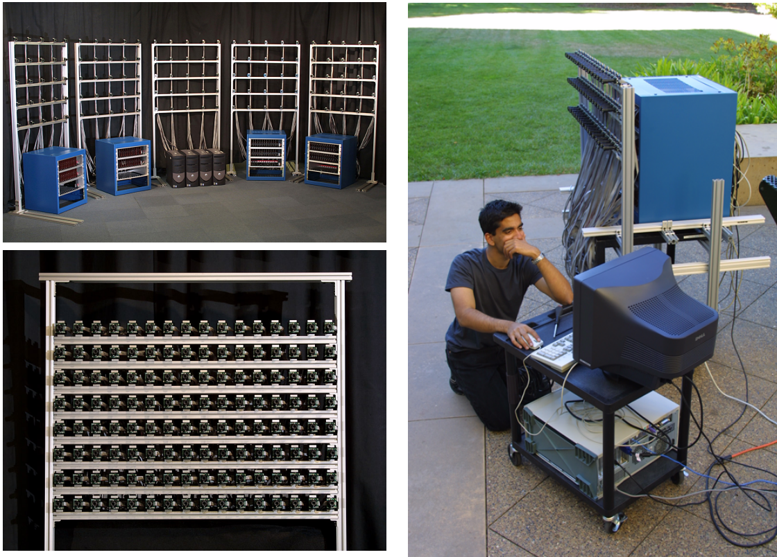
Figure 3.4: Different array configurations using 80/20 mounts.
