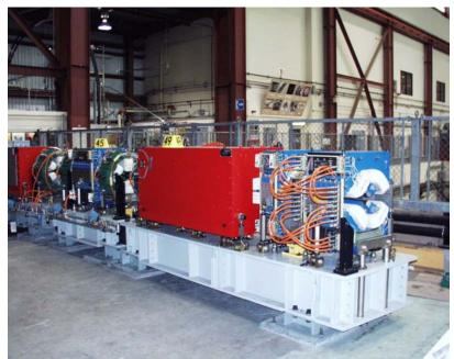
Standard Cell; 145D-T1 raft far left, 50Q raft (#45), and 145D-T2 raft (#49)
