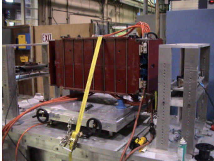
Magnetic measurement of the B8V magnet
