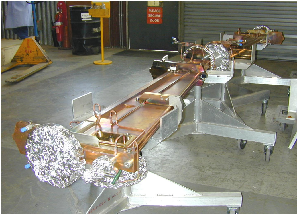
Figure 2.1: QFC Chamber – Final bake out and water jumper assembly completed
