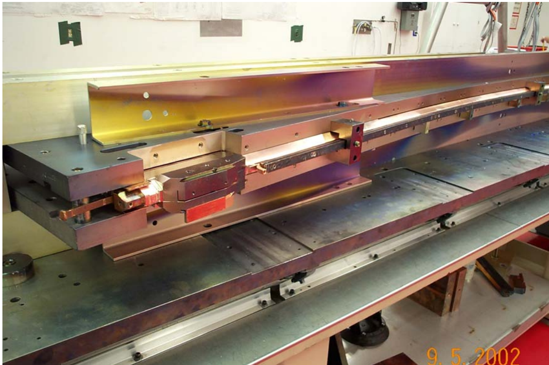
BM-2 Box Weldment Set-up and Eddy Current Break Weld Set-up
