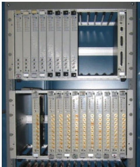
Some Low-level RF VXI modules ready for final testing
