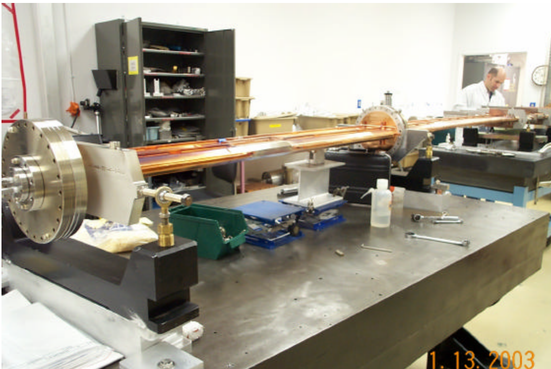
Figure 3 & 4: BM2-1 and BM2-2 Alignment and fiducialization of both chambers.
