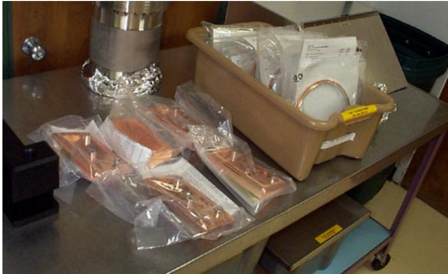
Figure 2.6: H2 Absorber Brazements and TSP Transition Brazements
