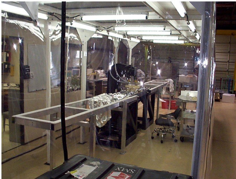
Figure 2.1: Clean straightening device/temporary clean room
