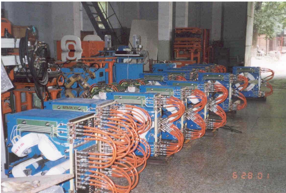
Completed Production Quadrupole magnets waiting shipment from IHEP
