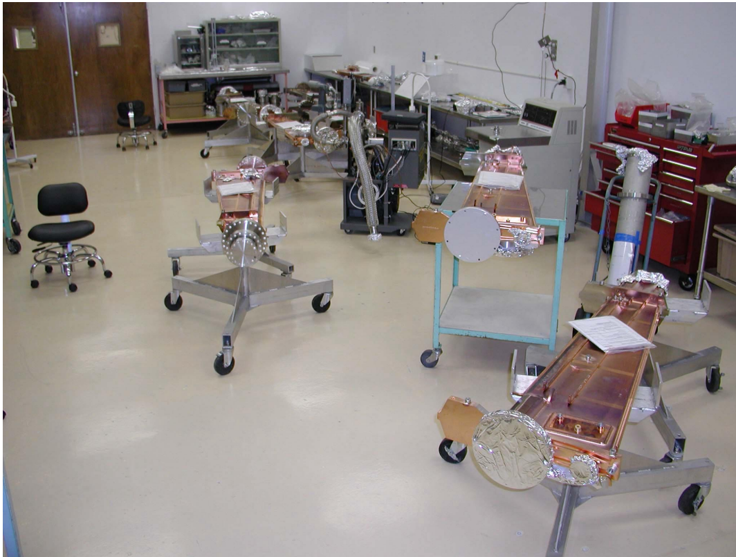
Figure 2: Completed QFC Chambers
