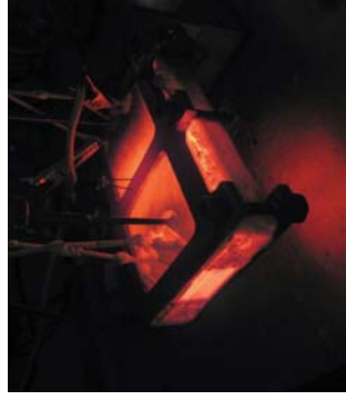
N 2 O decomposition cell: Yaniv Scherson and Brian Cantwell (2008)
