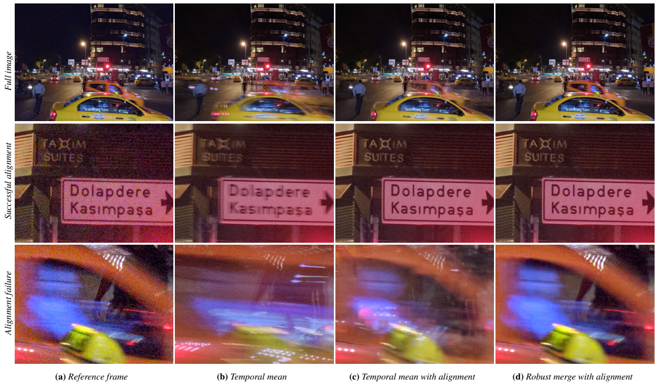
Figure 6: Merging 8 frames of a moving scene. The top row is the full image, the middle row shows a crop where alignment succeeds, and the bottom row shows a crop where alignment partially fails. (a) One frame from the burst is chosen as the reference. (b) Averaging all 8 frames without alignment produces ghosts in regions exhibiting motion. (c) Averaging with alignment eliminates ghosts in some regions (middle), but fails in others (bottom). When alignment is successful (middle row), the temporal mean resembles the reference; however, when alignment fails (bottom) the mean is different from the reference frame, leaving ghosts. (d) The result of our robust merge closely resembles the reference frame even when alignment fails. Despite alignment failure, some features are partially denoised. Note the yellow roof light in the foreground and the person in the background.
