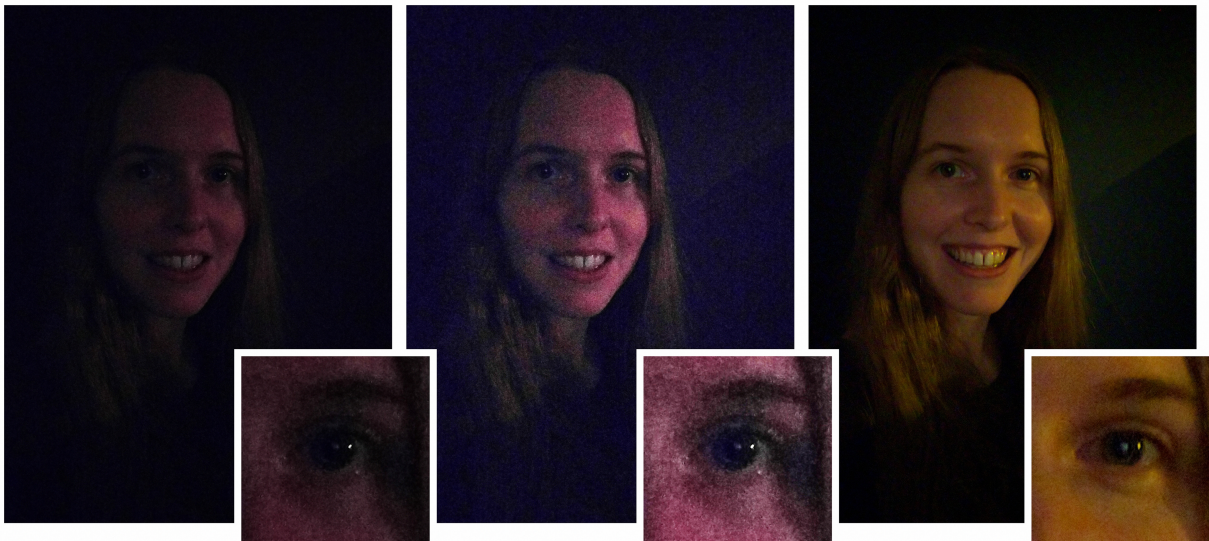
Figure 1: A comparison of a conventional camera pipeline (left, middle) and our burst photography pipeline (right) running on the same cell-phone camera. In this low-light setting (about 0.7 lux), the conventional camera pipeline under-exposes (left). Brightening the image (middle) reveals heavy spatial denoising, which results in loss of detail and an unpleasantly blotchy appearance. Fusing a burst of images increases the signal-to-noise ratio, making aggressive spatial denoising unnecessary. We encourage the reader to zoom in. While our pipeline excels in low-light and high-dynamic-range scenes (for an example of the latter see figure 10), it is computationally efficient and reliably artifact-free, so it can be deployed on a mobile camera and used as a substitute for the conventional pipeline in almost all circumstances. For readability the figure has been made uniformly brighter than the original photographs.
