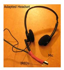
Figure 1. The adapted headset, with IREDs.
