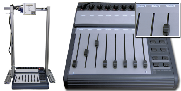
Figure 6. An external controller enables rapid surveying of multidimensional spaces. Variable names are displayed on top of assigned controls to facilitate mapping.
