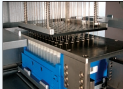
Septum Tube Stripper Plate Secures septum tubes in rack when removing fixed tips.
