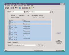
Sequencing protocols: Any number of detection methods and ambient temperature incubations can be sequenced in any order, enabling time-course protocols that can read a set of plates, store them in a magazine and then read the set again. It also enables assays using three or more fluorophores.
