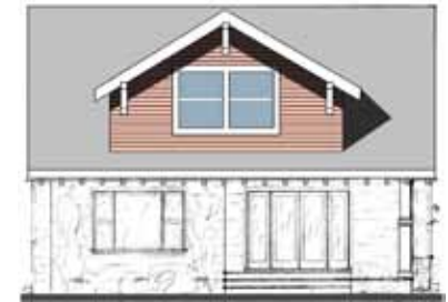
Avoid over-sized gable dormers like this
