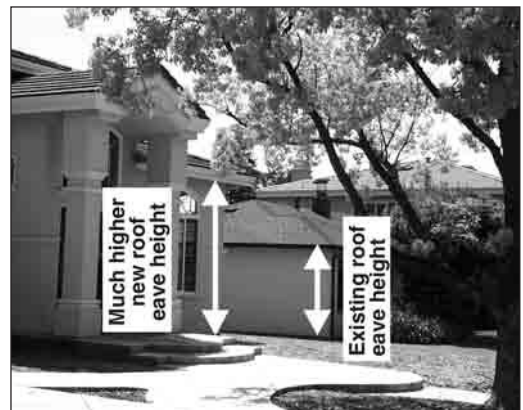
3.5.E Avoid large disparities in new roof eave heights compared to adjacent homes
