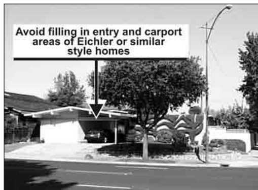
3.3.J Maintain distinctive carports and entries on Eichler and similar style homes
