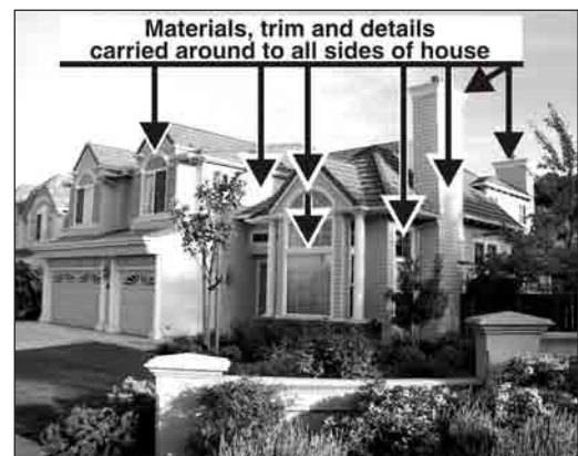
3.7.C Carry materials and details around to all facades of the house
