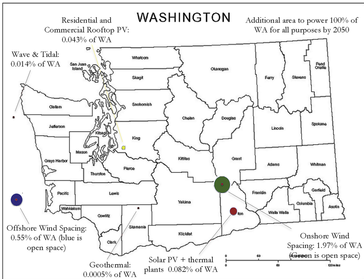
Fig. 1. Spacing and footprint areas needed for new plants and devices from Table 2 to repower Washington State for all purposes in 2050. The dots do not indicate the actual location of energy farms. For wind, the small red dot in the middle is footprint on the ground (not to scale) and the green or blue is space between turbines. For others, footprint and spacing are the same. For rooftop PV, the dot represents the rooftop area needed. (For interpretation of the references to color in this figure legend, the reader is referred to the web version of this article.)
