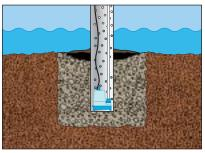
Pump from a settling pit: At the dewatering site, dig a small pit and fill with fine gravel. Pump through a perforated pipe sunk partway into the gravel.
