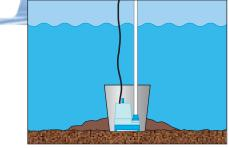
Using a submersible pump, pump from a bucket placed below the water level.
