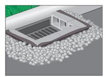
For large projects involving significant amounts of sediments or a steep slope, surround storm drain with a filtering dam. Water filters into storm drain through 1) crushed rock, surrounding 2) concrete blocks wrapped with filter fabric.
