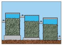
Direct water through a series of drums filled with successively finer gravel and sand.
