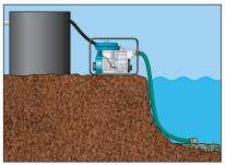
Pump from a Baker tank or other tank with sampling port(s).
