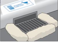
Place burlap bags filled with drain rock along the curb and around the nearest storm drain.
