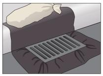
Cover storm drain with filter fabric, anchored under grate and above drain.
