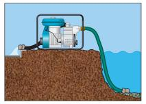
Wrap end of suction and discharge pipes with filter fabric.
