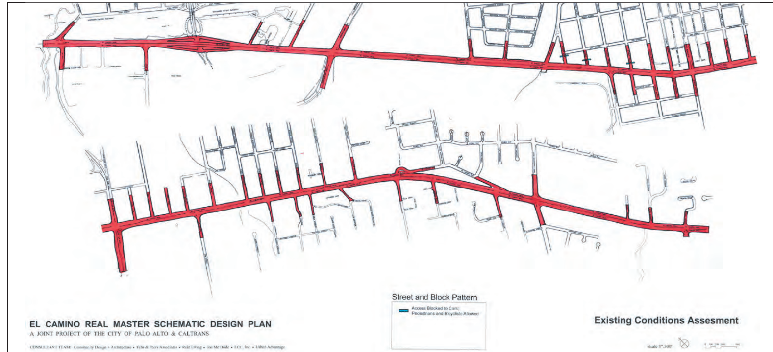
Figure 4.8: Street and Block Pattern. Note the frequency of T-intersections throughout the corridor
