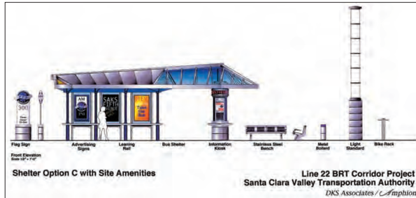
Figure 5.25: Conceptual illustration of VTA BRT amenities (November, 2001 - DKS Associates/Amphion)
