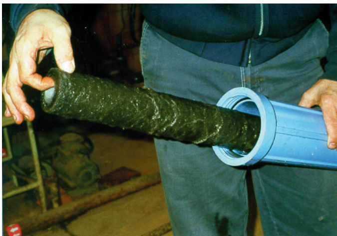
Figure 5.2 Clogged Prefilter (EPA, 2003).
