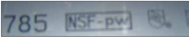
Figure 3.3 NSF-Approved PVC Pipe for Potable Water Use
