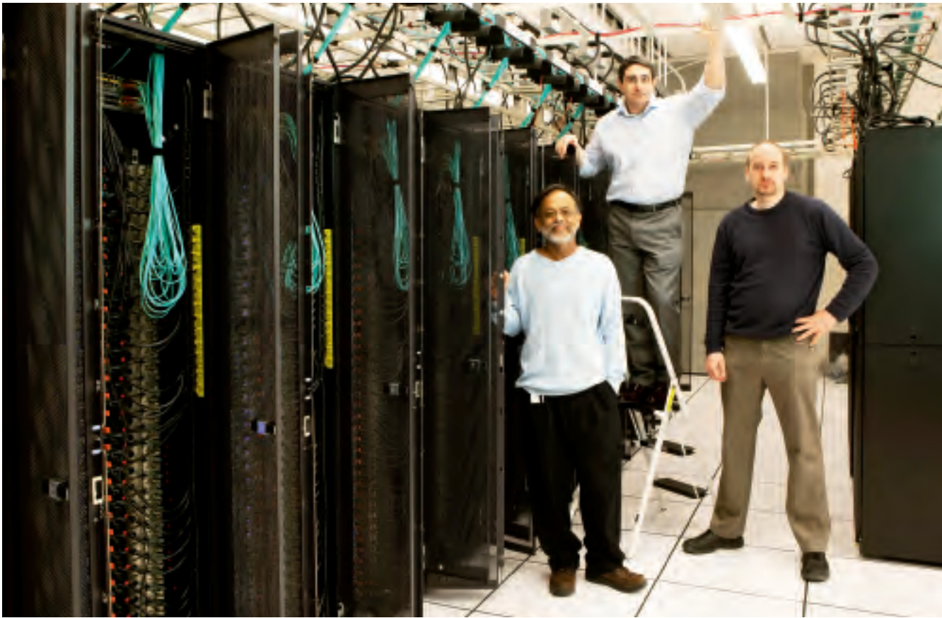
Janelia's IT team—Vijay Samalam, Spartaco Cicerchia, and Goran Ceric—recently updated its computing cluster, building it from commercially available hardware components by Intel, Dell, and Arista Networks, and using popular and now faster Ethernet networking.
