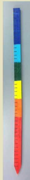
1 m stakes with 2 cm tallies are placed in the ground at the field site
