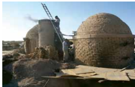
A traditional brick kiln (left) and an improved kiln design (right) operating in Mexico.
