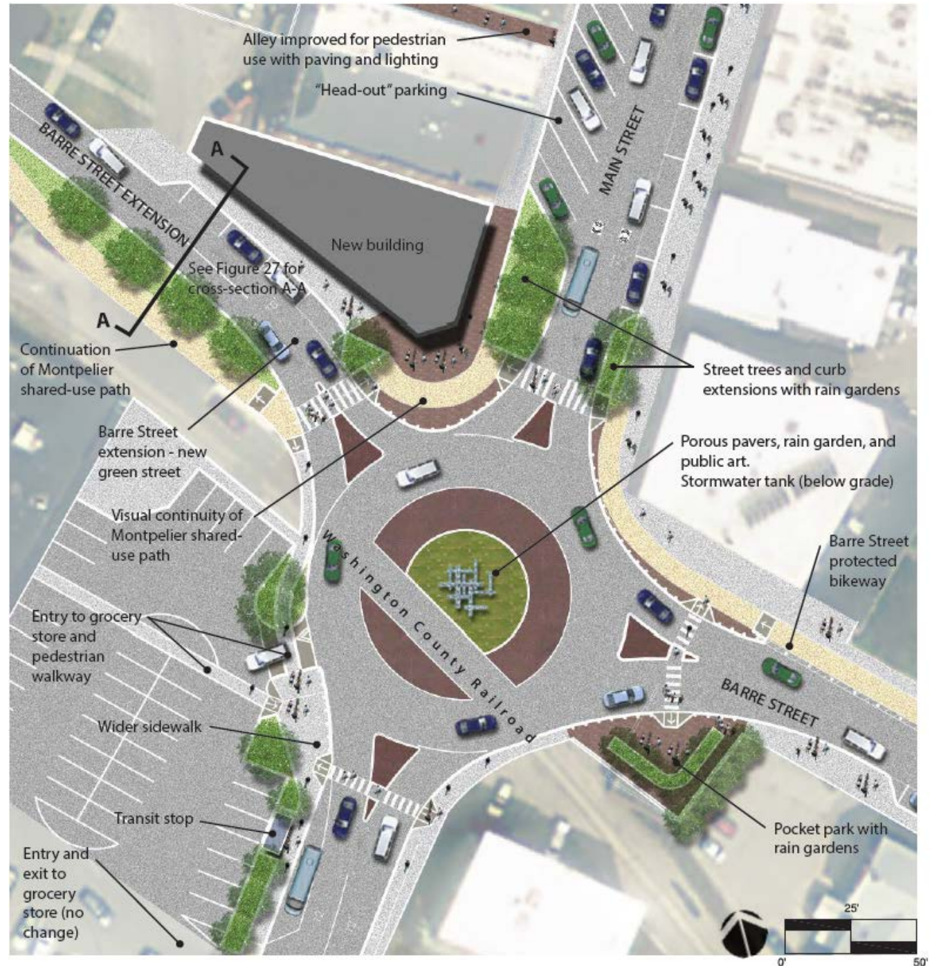
Figure 26: Design option for a roundabout at the intersection of Barre Street and Main Street.
