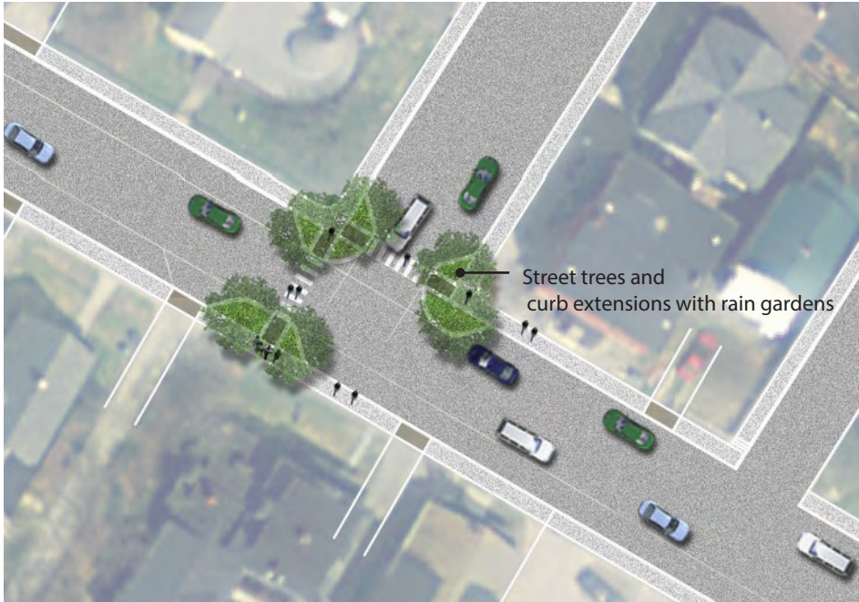
Figure 21: Plan for a typical enhanced pedestrian crossing with curb extensions and rain gardens.
