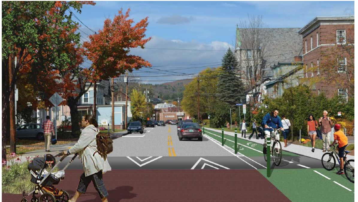
Figure 25: Design option for Barre Street with a protected bikeway, mid-block crossing and rain gardens.
