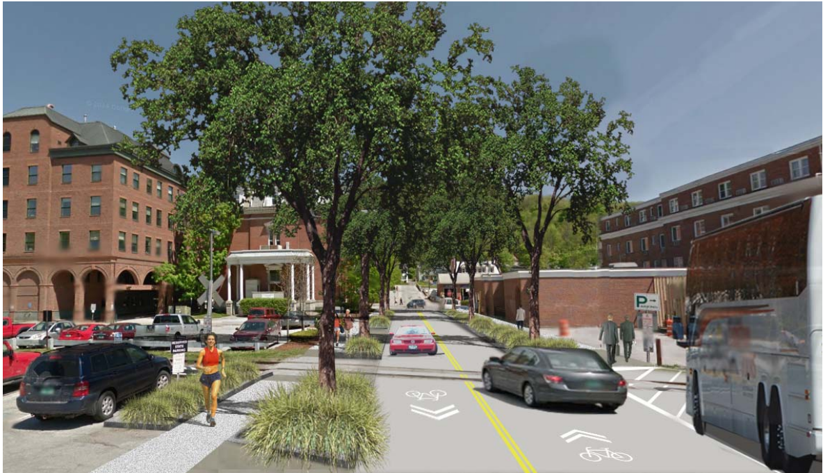
Figures 37: Design option for Taylor Street with sidewalks, "sharrows," street trees, and rain gardens.
