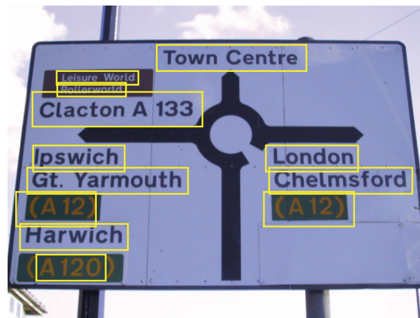
Figure 3.7: Estimated bounding boxes from text detector after all post-processing steps. There are two things to notice. First, the bounding boxes capture groups of words such as Leisure World or Town Centre . Word-level segmentation is done during end-to-end integration. Secondly, words that appear on the same “line” such as Ipswich and London are split into two boxes because of the large gap between the last character in Ipswich and the first character in London .
