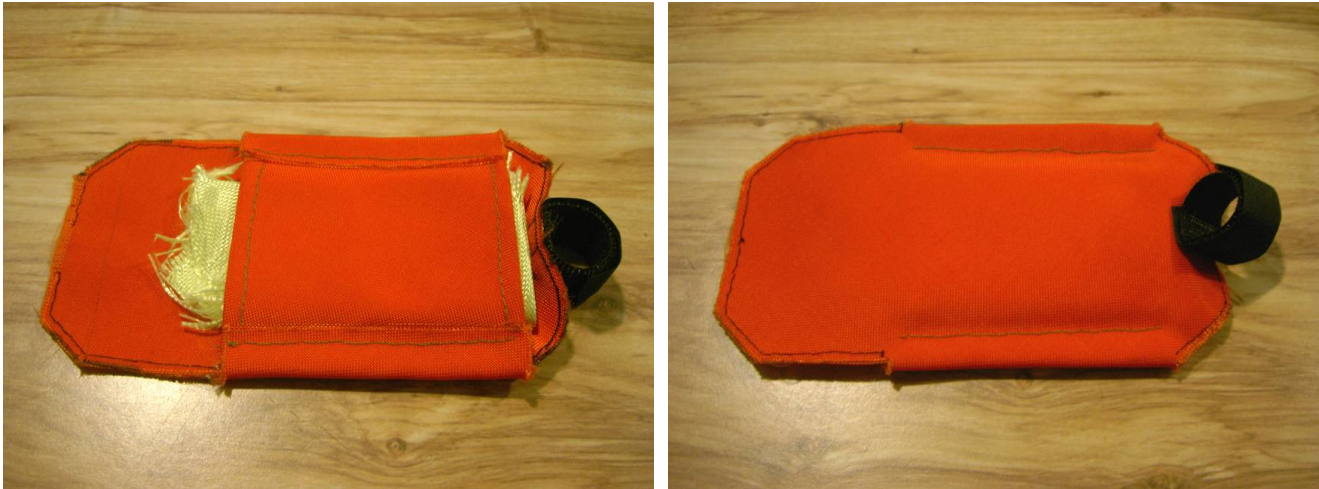
Picture 4: Handshield design for the clipper. From top left clockwise: the back view, with the pouch visible; the front view; the handshield incorporated into the clipper; the handshield in actual use.
