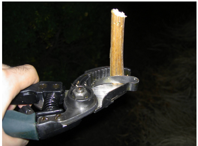
Picture 7: Pictures from field tests. From left to right: a depiction of branches classified as thin and thick, with a pen as a reference; a cantilever spring gripper is demonstrated with the Corona CH7720 pruner.
