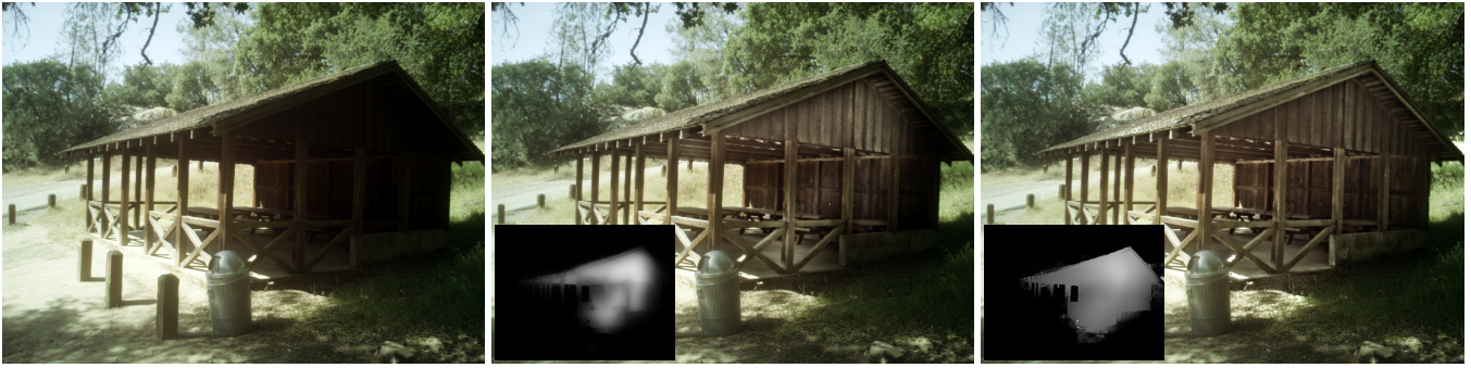
Figure 4: Improving edit mask quality offline. Left: An unedited viewfinder frame (from our tablet implementation), which has already undergone HDR blending and global tonemapping. Middle: The viewfinder frame with edits made by the user, displayed live. In this example, the user has brightened the unlit side of the building. Right: The final output after additional offline processing. The insets in the middle and right images show the computed mask before and after offline refinement. In the refined version, the selection is more homogeneous and its edges are sharper. While imperfect, the real-time result in the middle is sufficient to give the user a feel for the final output.
