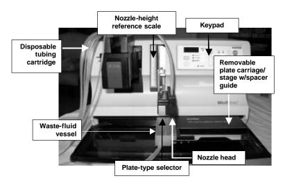
The components shown in the following figure are provided with the WellMate base unit.
