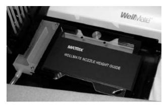
4. **Optional**: Peel the covering off the adhesive tape on the back of the nozzle-height reference scale and attach it to the instrument, to the left of the plate-type lever. When you have
