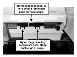
2. If the stage is not level with the nozzle tips, first try pushing the stage toward the back of the unit to ensure that it is
