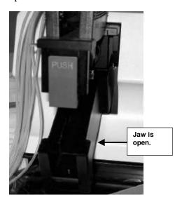
3. When installing the tubing, place the left-hand tube holder onto the arm first. Then place the other holder into position. Rotate the arm so the tubing is set into position.
