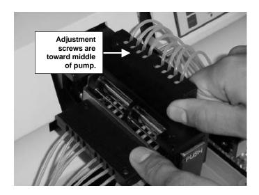
4. Push the cover on the pump mechanism to the closed position.
