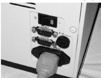
Turn the instrument on by pressing the power switch on the back of the instrument to ON.
