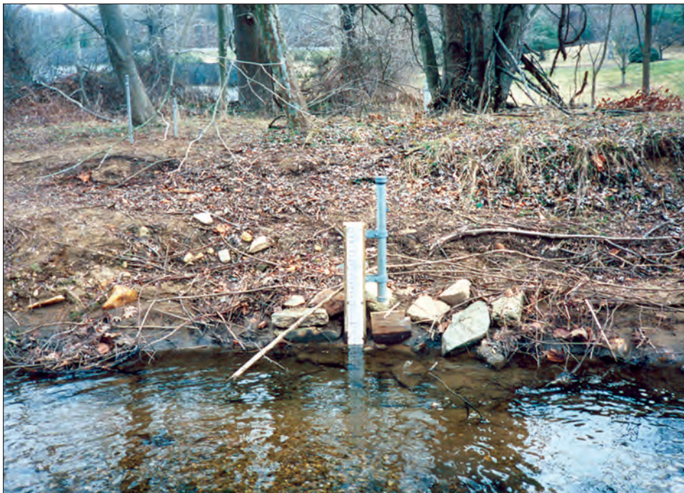
Figure 13. Crest-stage gage for obtaining high-water marks in the Minebank Run study reach. (Photograph by Edward J. Doheny, U.S. Geological Survey.)
