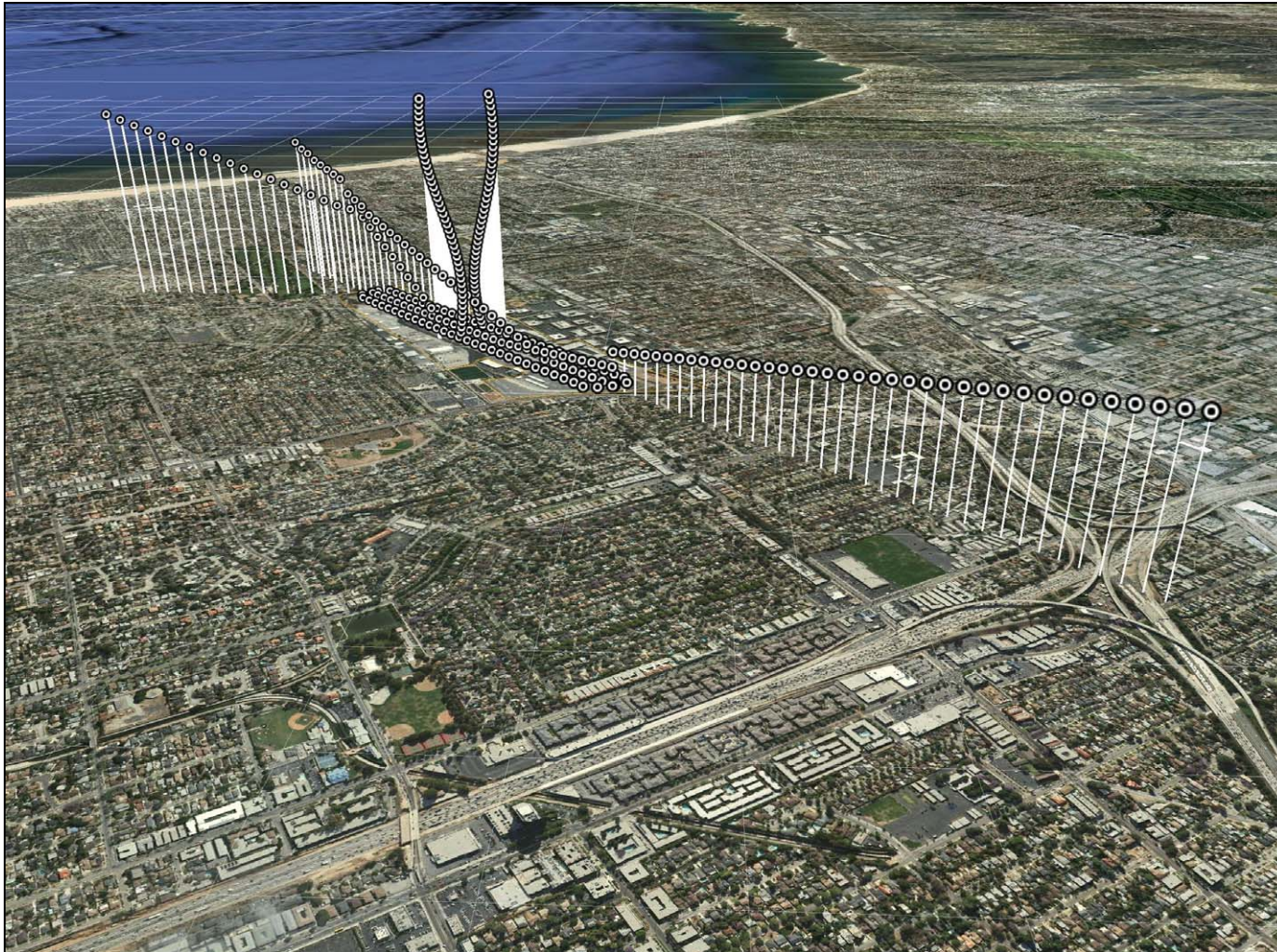
Figure 4-4. The Horizontal and vertical positions of emissions from fixed wing aircraft and helicopters (view is towards the west).
