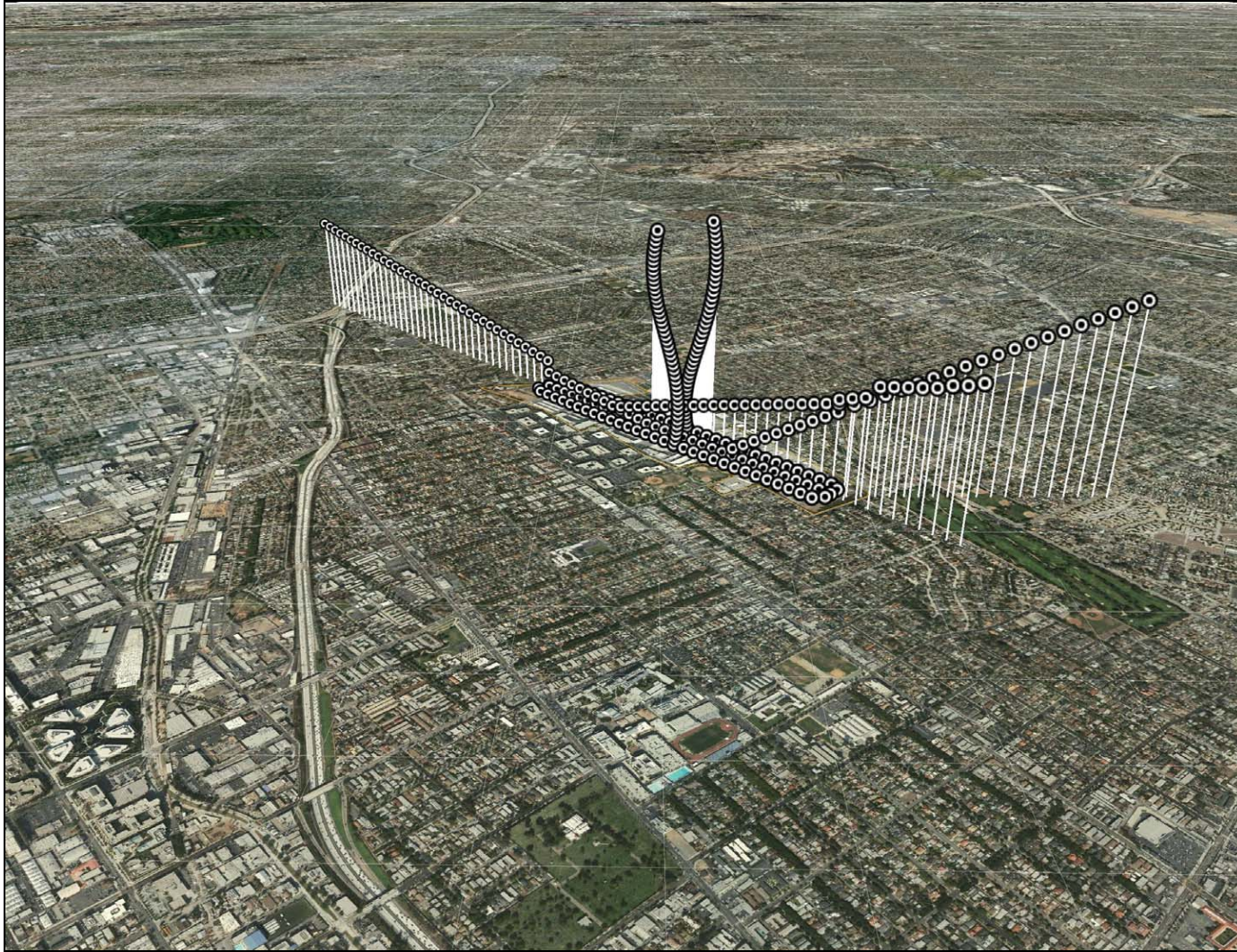
Figure 4-3. The Horizontal and vertical positions of emissions from fixed wing aircraft and helicopters (view is towards the east).
