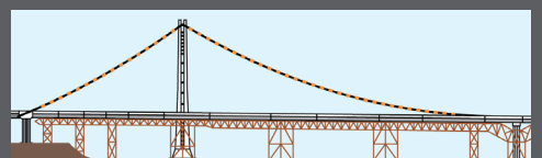
INSTALL CABLE BANDS
