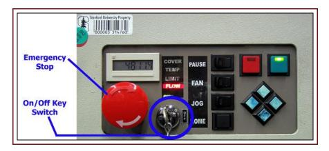
When the LaserCAMM first turns on, it goes through an initialization sequence and warms up its various components. Wait until the initialization completes (check status on the four-line LCD screen on the upper surface) before you start working with the machine.
