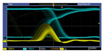
Digital phosphor technology enables a 5,000 wfm/s waveform capture rate and real-time intensity grading on the MSO/DPO2000 Series.
