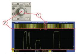
Wave Inspector controls provide unprecedented efficiency in viewing, navigating, and analyzing waveform data. Zip through your 1 Mpoint record by turning the outer pan control (1). Get from the beginning to end in seconds. See something of interest and want to see more details? Just turn the inner zoom control (2).
