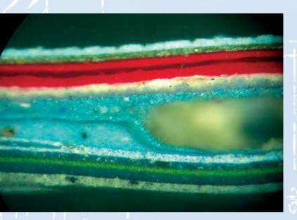
A microscopic cross section of paint layers on a car that was often repainted.
