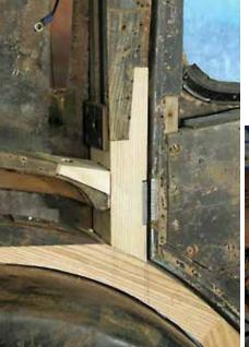
A restorer at Autoservice René Große planishes a large panel using a pneumatic hammer; the wooden frame of a Hispano-Suiza is given a partial restoration; this model for a Bugatti fender was made by laser-scanning an intact fender, flipping the image, and using a water-jet cutter.
