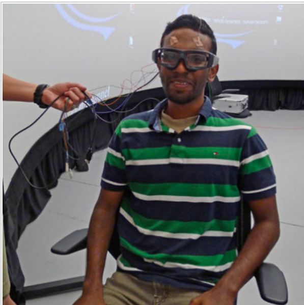
A researcher in Nass' lab is outfitted with eyetracking glasses, EEG sensors and skin conductance sensors ahead of his drive in the simulator.
