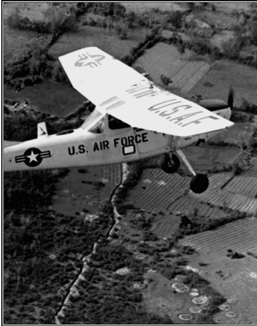
A US Air Force O-1 observation plane, shown here overflying South Vietnam. The aircraft was used throughout Southeast Asia to spot, target, and evaluate strikes on enemy forces. US Air Force photo.
