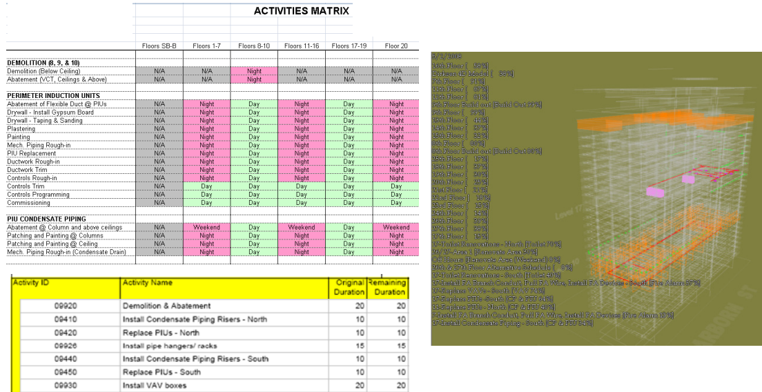
Figure 6. The traditional planning methods used on TC#2 included a CPM schedule, day/night/weekend activities matrix, and 4D Model.
