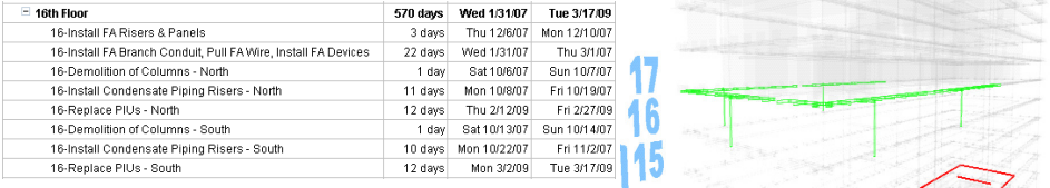
Figure 7. The current representation of the project schedule and 4D model of the condensate piping activity does not allow project managers to distinguish the impact of construction workshifts on tenants.
