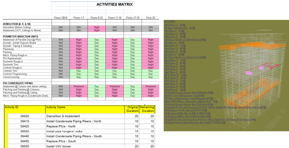
Figure 19. The traditional planning methods used on TC#2 included a Primavera schedule, day/night/weekend activities matrix, and 4D model
