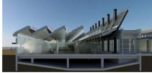
Figure 10: A new US border station located in New Mexico will be the first federal NZE building. The figure shows the proposed solar chimneys that provide natural stack ventilation during the day through the basement thermal reservoir and allow for night flushing to pre-cool the building. (Image courtesy of Richter Architects)
